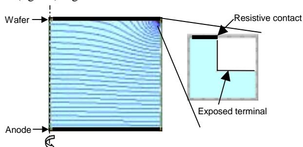
Fig. 2: Computer simulation (CELL-DESIGN<sup>®</sup>) of copper deposition on a wafer (top) through a resistive (0.25 ohm) contact. Axi-symmetric cross-section is shown with center of the wafer on the left and the resistive contact at the wafer circumference (top right). Inset shows contact details. Equi-potential lines, 14 mV apart are shown.
