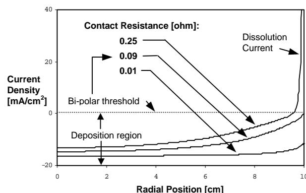
Fig. 3: Current distributions across a wafer plated through a resistive contact (Fig. 2). Dissolution near the edge is evident for the 0.25 ohm contact resistance. The bi-polarity threshold is 0.09 ohms. The effect of contact resistance on the deposit uniformity is noted.
